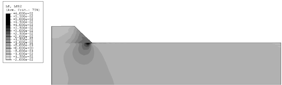
FIGURE 4.27 Distribution of shear strains at the end of construction of layer 3: elapsed time, 6 days.
